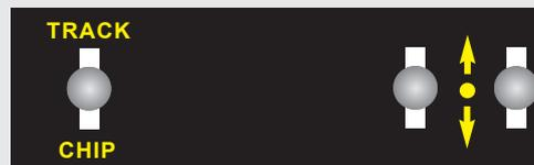
The **track driving handles** are to the right on the tracking control panel marked with arrows. The left handle is for the left track and the right one for the right track. They are spring loaded to the stop position, and proportional. The more you push the handles, the faster the chipper moves to a maximum of a walking pace.
